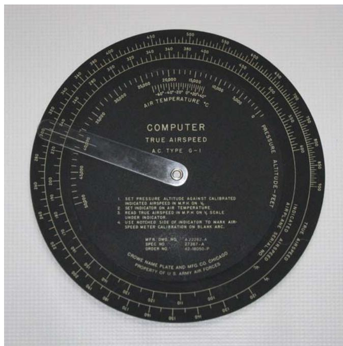
flight level pressure altitude and flight level air temperature. One could argue that the E-6B could have easily provided a bombardier with true airspeed values, but keep in mind that the G-1 is a single purpose flight computer, a full eight inches in diameter, with well-marked and well-spaced lines and numbers. As well, all markings were applied with good old-fashioned radium-based “radioactive” luminescent paint on a black background, so the computer could pretty much be used in the dark!
